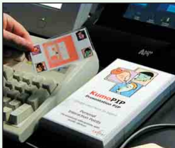
Figure 5: A user logs into an embedded PIP interface by swiping their RFID card.
